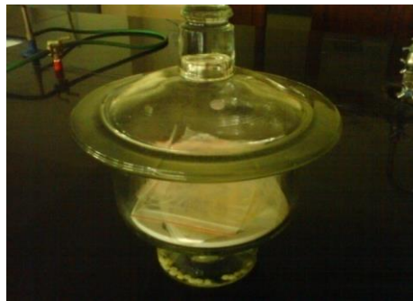
Fig 6: Storage of the prepared patch at dry condition.
